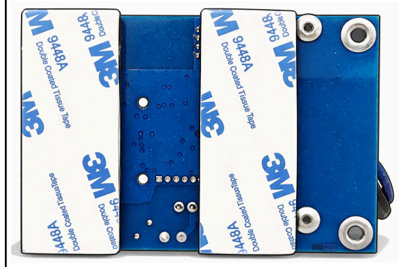
Figure 28. Adhesive strips on the TPG015 gateway board
