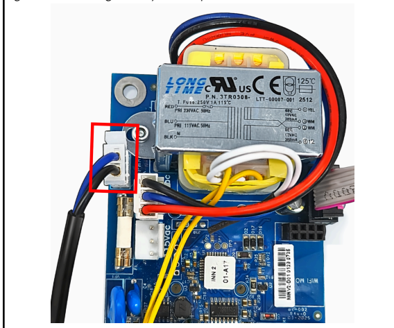
Figure 21. TPG015 gateway board power connection
