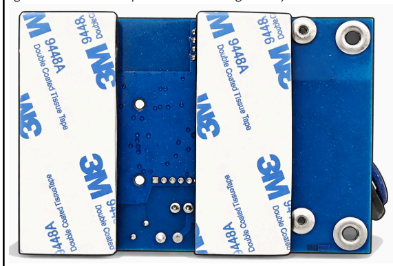
Figure 8. Adhesive strips on the TPG015 gateway board
