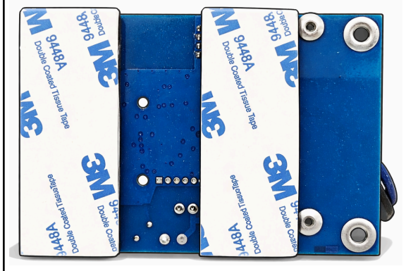
Figure 50. Adhesive strips on the TPG015 gateway board
