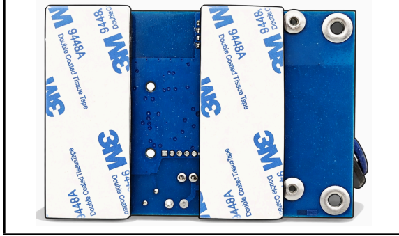
Figure 68. Adhesive strips on the TPG015 gateway board
