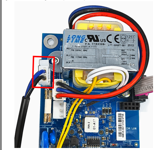
Figure 80 TPG015 gateway board power connection
