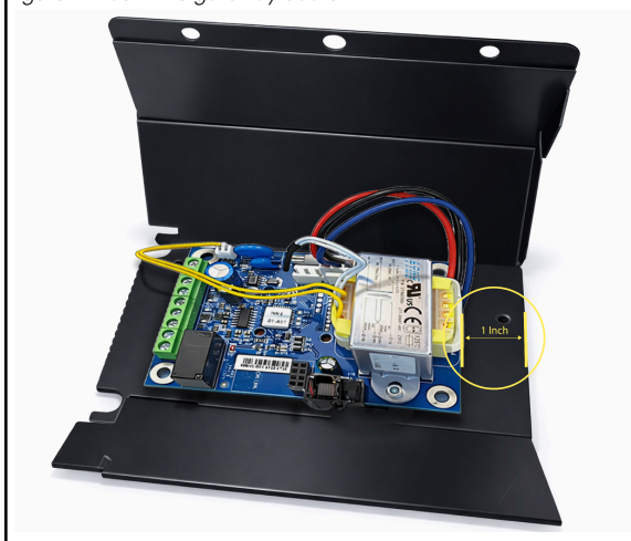
Figure 9. Mount the gateway board
