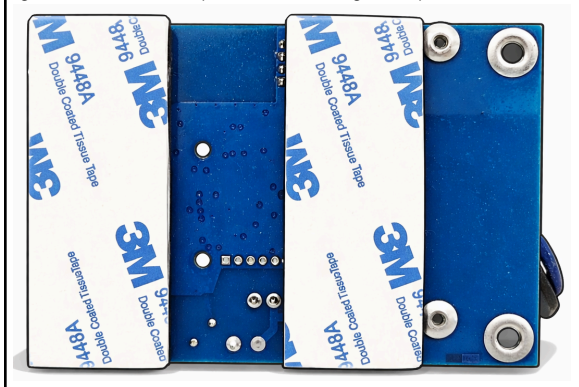
Figure 88. Adhesive strips on the TPG015 gateway board
