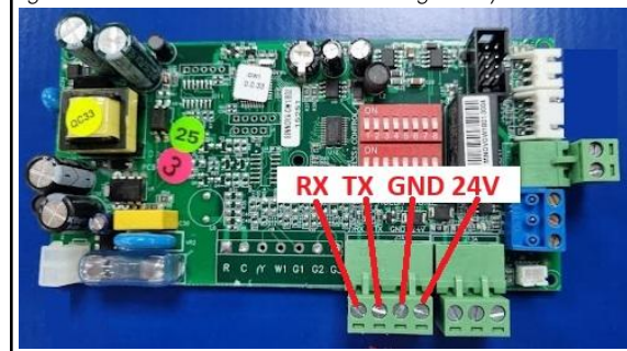
Figure 1. Connect control cable to the GW1 gateway
