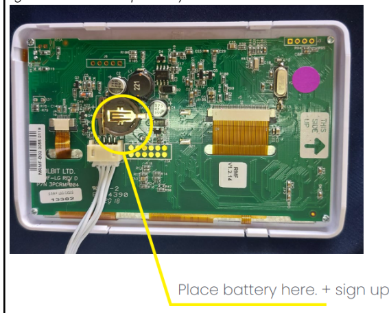
Figure 8. Install Backup Battery
