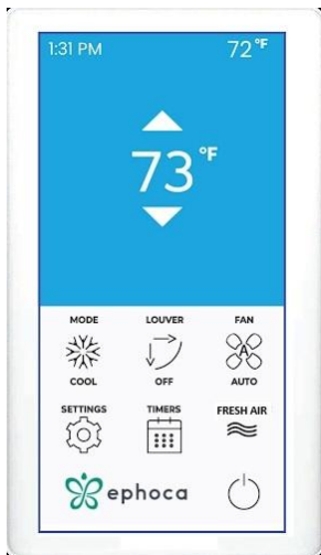
Figure 13. TFTH20 controller Home screen
