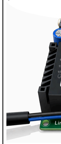
Figure 46. Connect the communication cable to the gateway board
