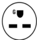
NEMA6 250V receptacle for 208/230V
