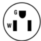
NEMA5 115V receptacle for 115V
