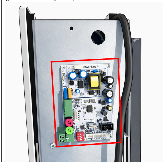
Figure 38. Mount the gateway board
