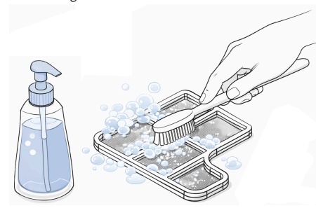
Figure 27. Cleaning the filters
