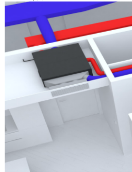
Figure 11. Shared supply and exhaust vents
