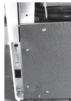
Figure 4. Insert the male connector
