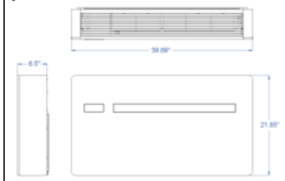
Figure 9. Wall Mounted Standard Dimensions
