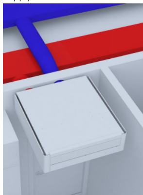
Figure 6. Shared supply and exhaust vents
